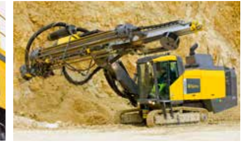
When equipped with the standard feed option, the FlexiROC D60 and D65 are both capable of handling an even wider range of drilling angles with ease.
