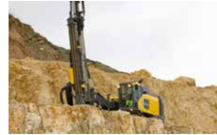
Built for high efficiency mining, the DTH hammer benefits from a precisely matched compressor.
